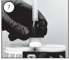
Secure the Static Mixer and Backflow Restrictor to the cartridge by slipping the Nut over the Static Mixer. Screw the Nut firmly to the cartridge.
