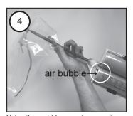
Using the cartridge pouch, purge the air from one side of the cartridge. Pointing the tip at an upward angle into the pouch, squeeze the trigger until all the air is out of the lower tube
