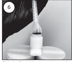
Slide the Static Mixer over the top of Backflow Restrictor and the rim of the cartridge.
