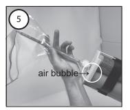
Flip the cartridge over and repeat step 4 to purge the air from the other tube. Once the air has been purged, point the cartridge downward or horizontally to prevent mixed Flash Floor from flowing backwards into the cartridge
