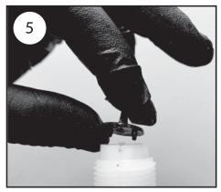
Insert the Backflow Restrictor into the mouth of both sides of the cartridge. Make sure the 2 holes in the Flow Restrictor are lined up with each opening of the cartridge.
