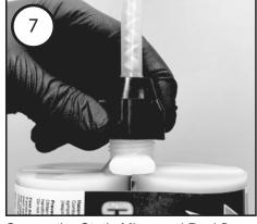
Secure the Static Mixer and Backflow Restrictor to the cartridge by slipping the Nut over the Static Mixer. Screw the Nut fimly to the cartridge.
